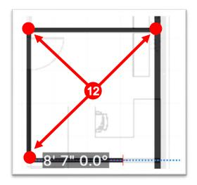
Note: Dimensions during drawing are from the center of the wall, as the walls have thickness. Once you complete the wall, it will display the interior or exterior dimension accordingly. You can adjust all walls by either clicking on the wall and dragging the entire wall, or by clicking on the end of the wall and moving it.
